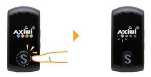
\* This function is to allow a follower mode device to cancel its permission to speak by the user himself/herself. When in normal "listening mode", only one LED for the specific channel on the unit will be blinking, instead of four lit LEDs.
